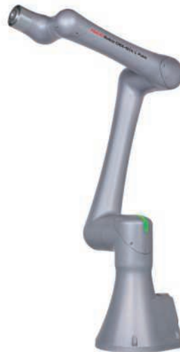
World's first EX-Proof Collaborative Paint Robot CRX-10iA/L Paint
