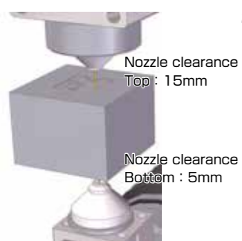
Dis steel, 40mm, φ0.25 brass wire, 1 rough 2 skims, Accuracy ±3μm, Roughness Ra 0.60μm
