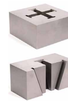
Die steel, 50mm, φ0.20 soft wire 1 rough 3 skims Taper angle 20 degrees
