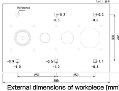
Die Steel, 30mm, φ0.20 brass wire 1 rough 4 skims, 20mm square holes Pitch accuracy: X -0.9 to 1.1μm, Y -1.0 to 0.0μm
