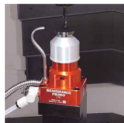
Tool length switch for automatic measurement
