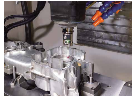
Example of measurement with High-speed SKIP
