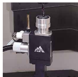
Tool length switch for automatic measurement
