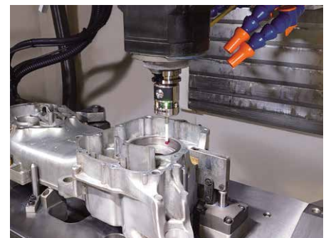
Example of measurement with High-speed SKIP
