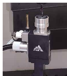
Tool length switch for automatic measurement
