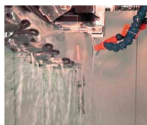
Cleaning unit for tool taper shank
