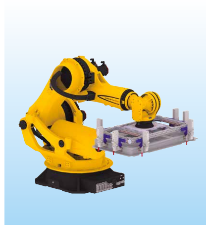
Battery Unit Handling (Transporting to backwards of robot)
