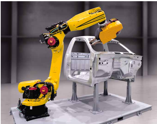
High Speed Spot Welding (Cable Integrated Arm)
