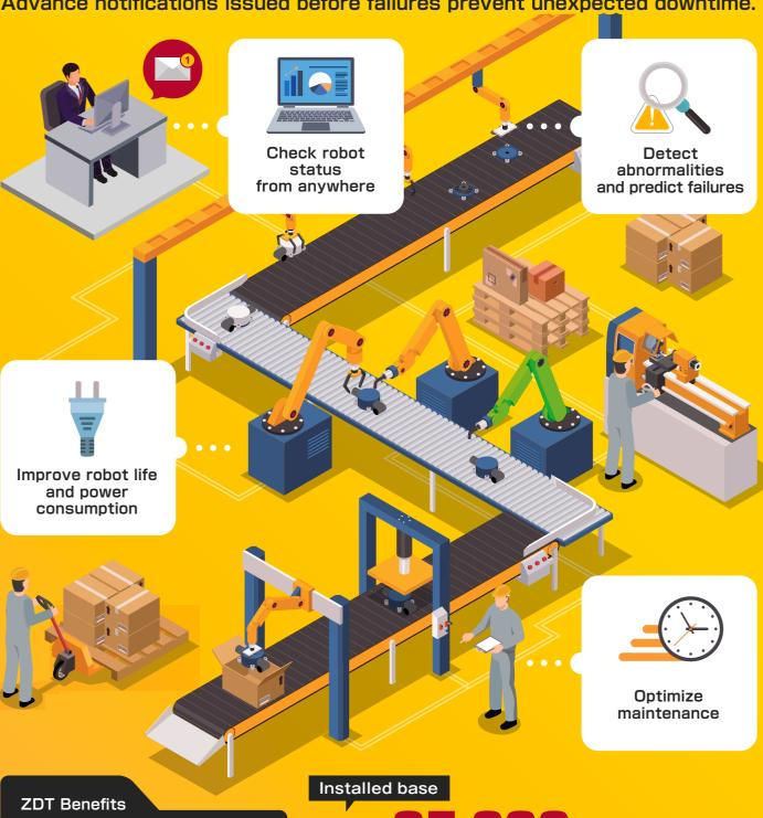
A single robot breakdown can cause significant system production downtime. ZDT includes analytics that can detect robot abnormalities and provide advance notification that action is required so maintenance can be performed to prevent unexpected downtime.
