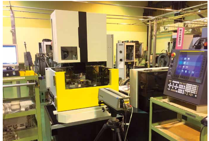
Automatic machine accuracy measurement system (laser length measurement)
