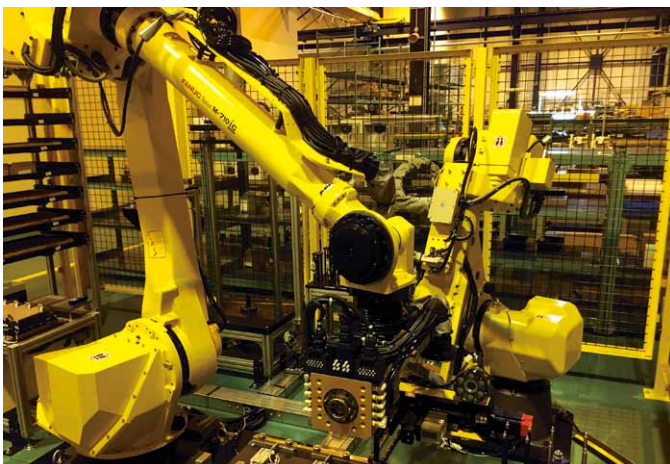
Automatic assembly system that performs multi-product production (Dielectric fluid draining unit, work-pan seal unit, etc.)
