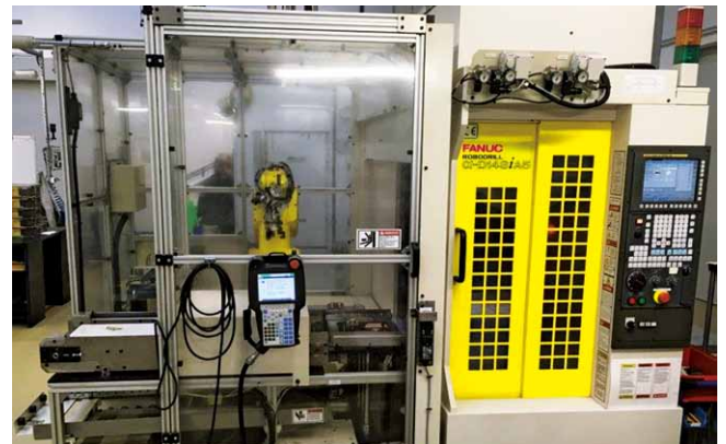
Installation of a system that combines the FANUC ROBODRILL and the FANUC robot (facility in the Czech Republic)
