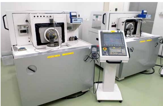
Mirror holder processing using the ROBOTANO \alpha -0iB (1st floor)
