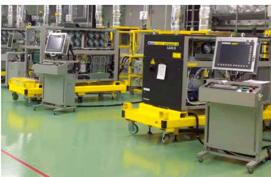
Automatic carbon dioxide gas laser test using the CNC (3rd floor)
