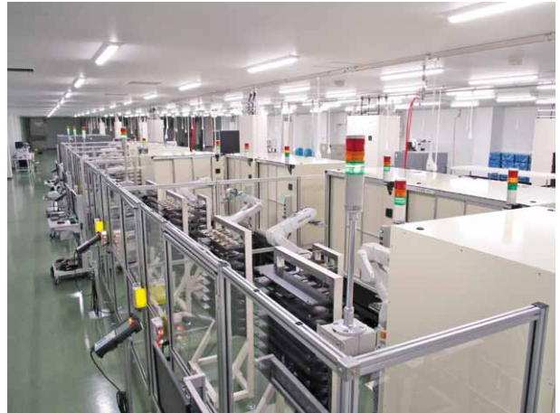
Automatic manufacturing line of LD modules by FF Laser Corporation (1st floor)
