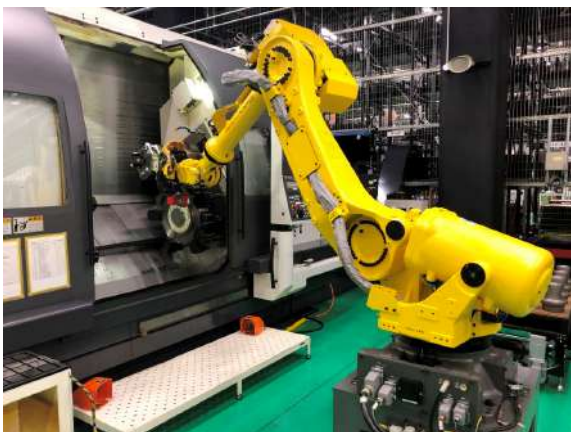
Automatic workpiece loading and unloading in a lathe
