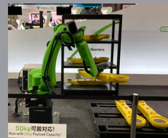
Transport of castings using a 50kg payload collaborative robot
