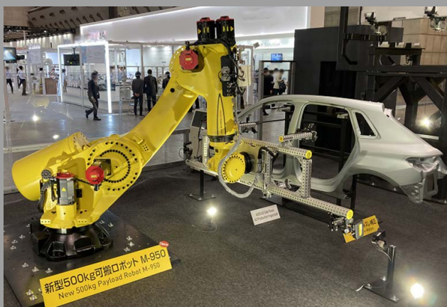
500kg payload robot transporting an automotive body panel
