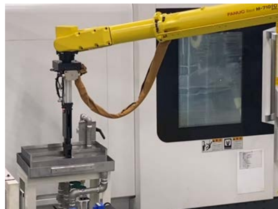
Simple pan for washing with water in the “shaft machining cell”
