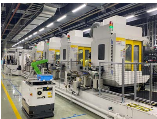
RocoMo-V supplying materials and collecting products
