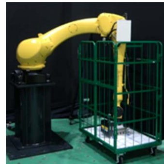
Approaching deep area utilizing the curved arm
