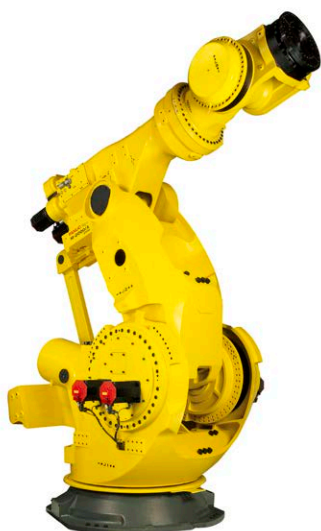
M-2000iA, the large 6-axes articulated robot with a maximum payload of 2.3 tons
